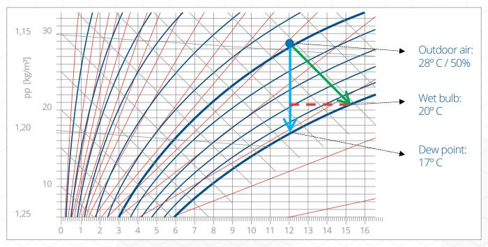
Please notice that the efficiency of the heat exchanger determines to which degree the lowest possible temperature (dew point or wet bulb) is achieved. A more efficient heat exchanger will bring the supply air closer to the ultimately possible temperature. In the ICECUBE, the evaporation process takes place on the surface of the exchanger, with an ideal distribution of the water over the exchanger surface. This is one of the reasons that the ICECUBE reaches the highest efficiency.
